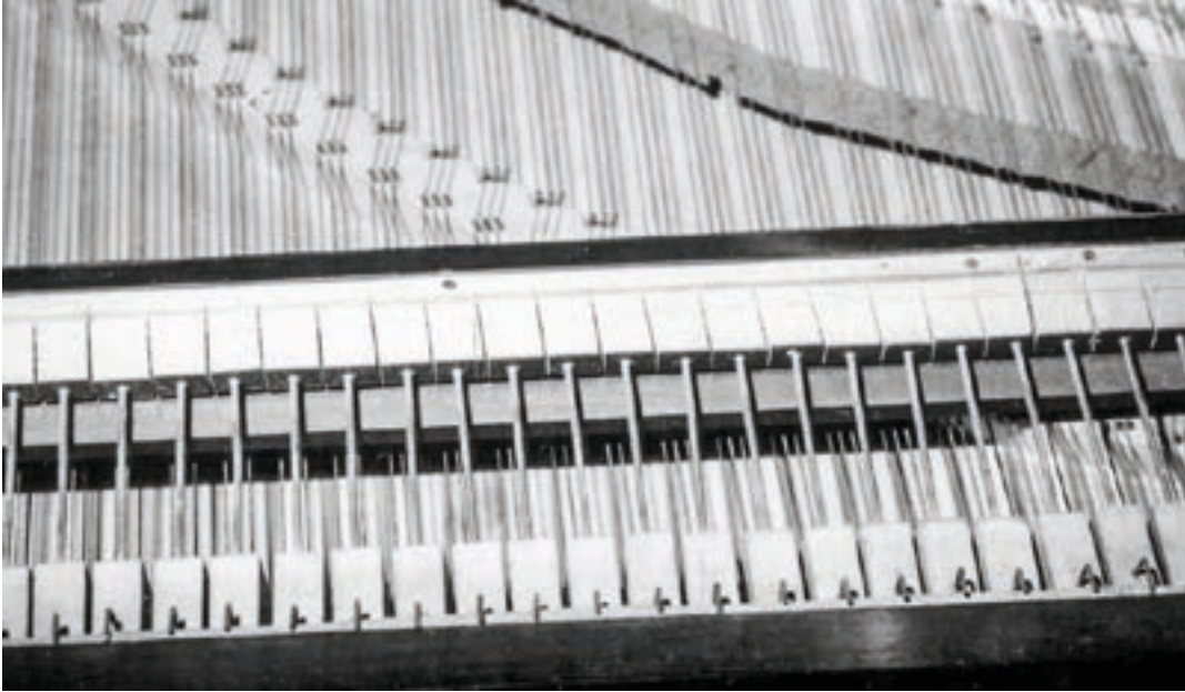
15 | Detail der regulierbaren Messinghäkchen an den Dämpfern in MÜNCHEN / Detail of adjustable brass hooks at the front end of the dampers of MUNICH
